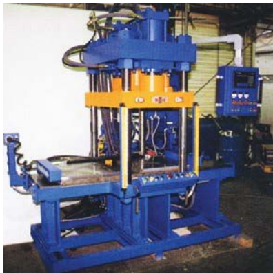
150-ton downacting transfer press with dual platen shuttle
