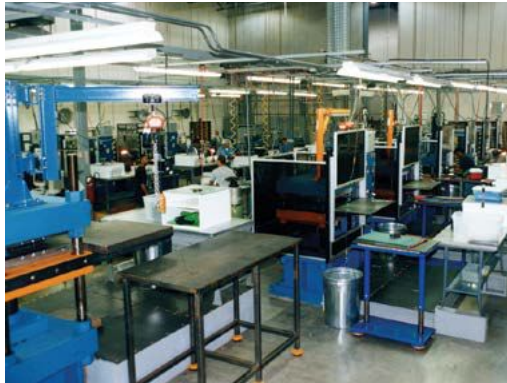
Installation of multiple Vantage compression molding presses
