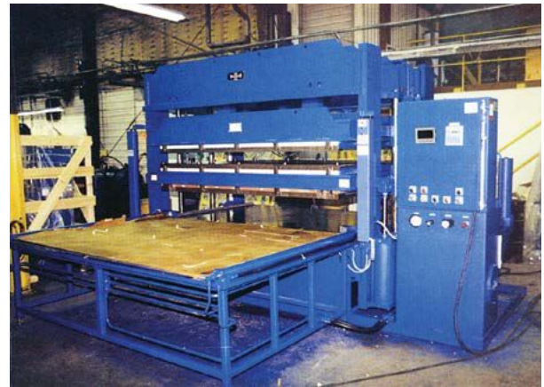
Molding press with 96" x 72" heated and cooled platens and lower platen shuttle
