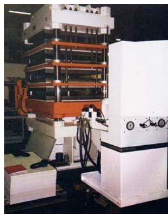
350-ton, 4-opening molding press with remote power unit
