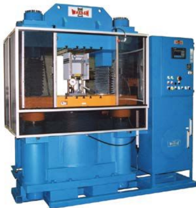
1000-ton compression press (12-ton Carver manual press shown in clamp)
