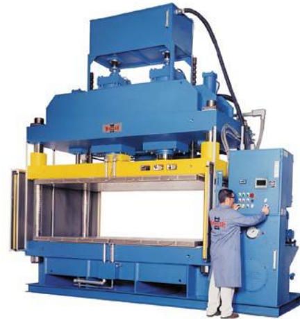
400-ton, down-acting press with 120" x 60" platens for composite panels
