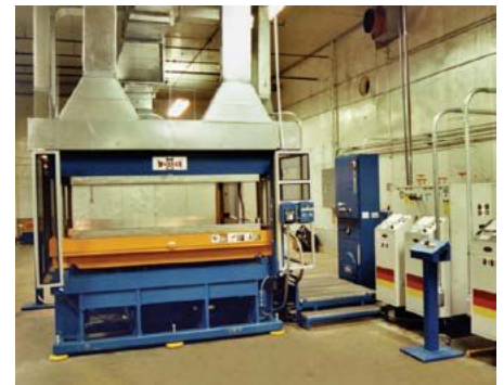
150-ton compression molding press with 96" x 72" multi-zone oil heated platens
