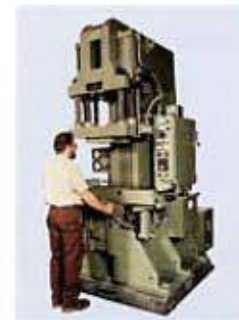
Custom C-Frame transfer molding press with shuttle table. Custom presses are available through your WABASH MPI representative.
