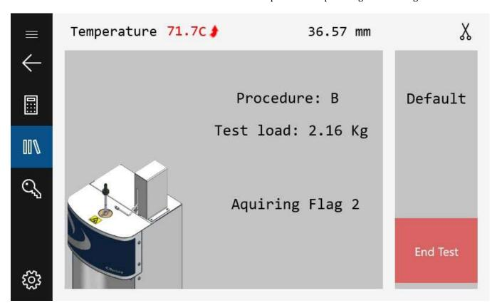
For each flag length, the LMI will measure the sample time interval that has elapsed.
