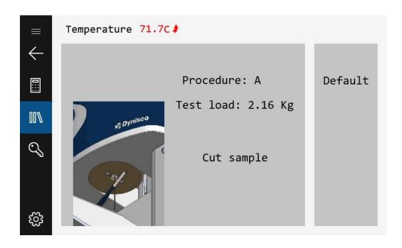
For each sample cut, the LMI will either cut (or prompt the user to cut) the sample after the sample time interval has elapsed. Ensure that the samples are moved away from the landing area, so samples don't fuse together.
