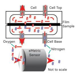
Systech Illinois' eMetric sensor analyzes 100% of the oxygen passing through the sensor resulting in unequivocal conformation of ASTM D3985.
