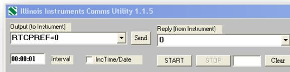
Connect the GS6000 to a computer using the USB cable provided. Start the Systech Illinois Client program. In the "Output (to instrument)" window, key in the preferable format with the command "RTCPREF=0" for DD/MM/YY format and click "send". The instrument will reply "0" as shown above indicating the acceptance of the command. The formats MM/DD/YY and YY/MM/DD can also be set with the commands "RTCPREF=1" and "RTCPREF=2" respectively.
